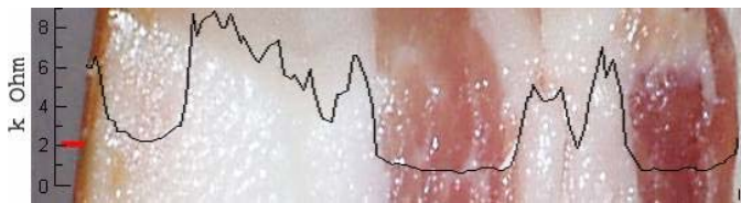
Fig.3 Measured modulus at 10 kHz plotted as a function of insertion depth in a piece of bacon. The red mark indicates the starting point of the horizontal needle insertion path.
